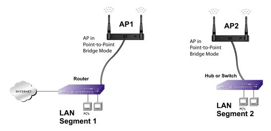
Figure 4-8 Wireless point-to-point bridge setup
